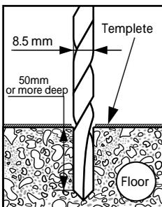
1. Drill the anchor holes of a specific diameter and depth.
