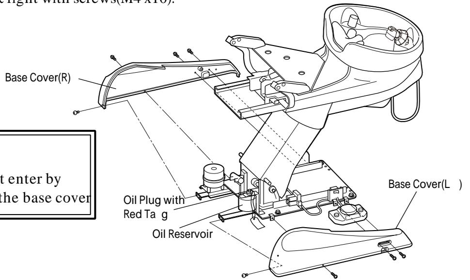
3. Fix the center base cover with screws and plastic washer (M5 x 20).
