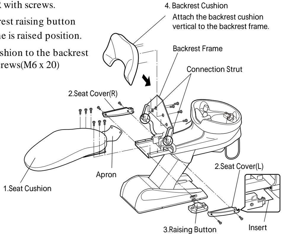
5. The apron from seat cushion is inserted between the backrest cushion and the cylinder, then fixed with two screws(M4 x 18)
