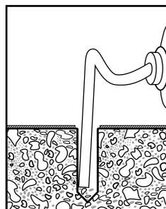
2. Clean each anchor hole thoroughly using a vacuum cleaner with a narrow nozzle attachment to reach into the hole and remove all debris.
