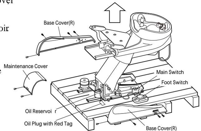
Note : Do not remove the unit from the pallet until the unit xing position is ready.
